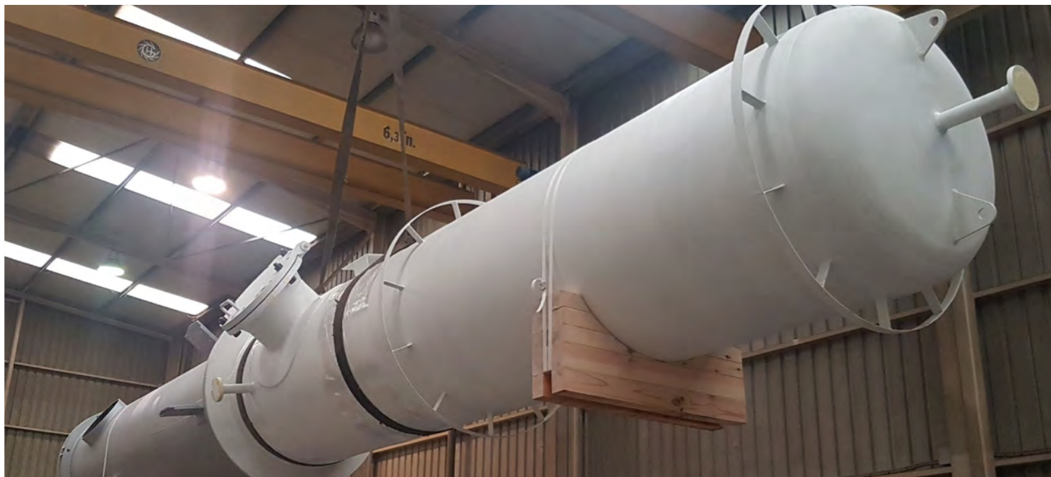
Weld overlay flash tank c.s. + 317L
