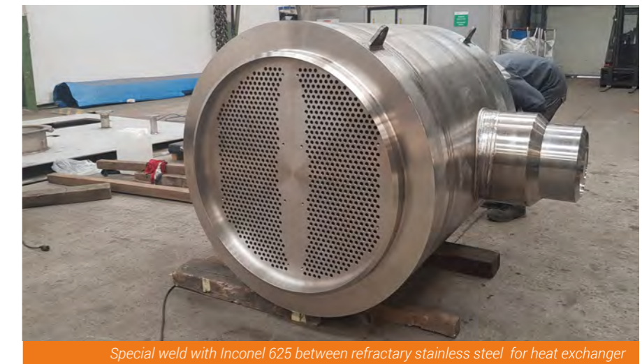
Special weld with Inconel 625 between refractory stainless steel for heat exchanger
