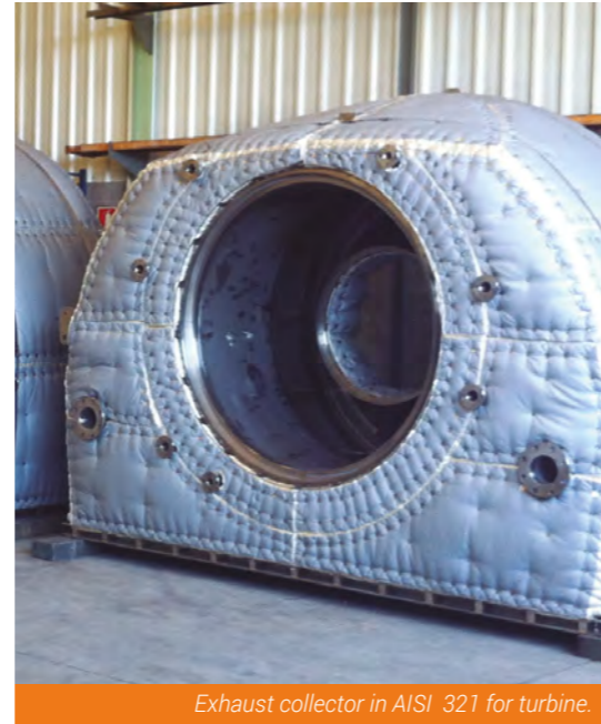
Exhaust collector in AISI 321 for turbine.
