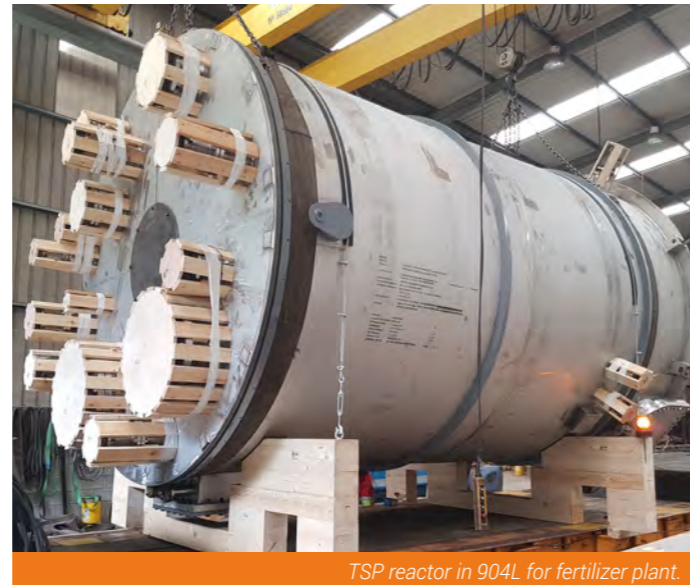
TSP reactor in 904L for fertilizer plant.
