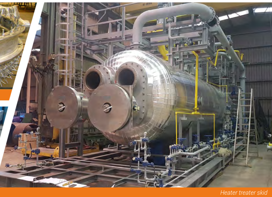
Heater treater skid
