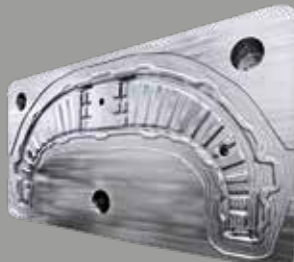
FORM PAD Material: Forged Steel Weight: 20 t
